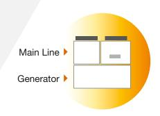
Redundancy increases uptime. i-FR-G04-Z extends this concept also to the electrical supply: the unit, equipped with an ATS\*, can be connected to two separate power lines to enhance the system's dependability.
